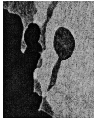
Fig. 4 Typical shadowgraphs of ligament base (turbulent) breakup at the surface of round and annular turbulent freejets in still air.
